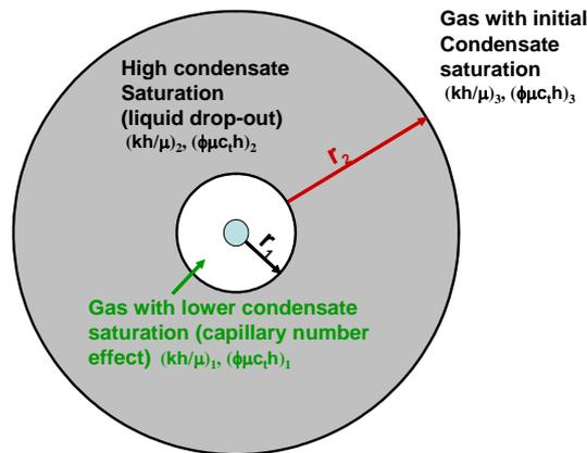
Figure 1: Schematic of three-region radial composite model
